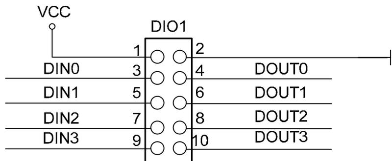
The 4-bit (bit0 ~ bit3) binary value represents the digital output signal.
