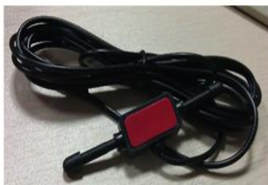
Figure 15: Example of a Dipole Antenna
