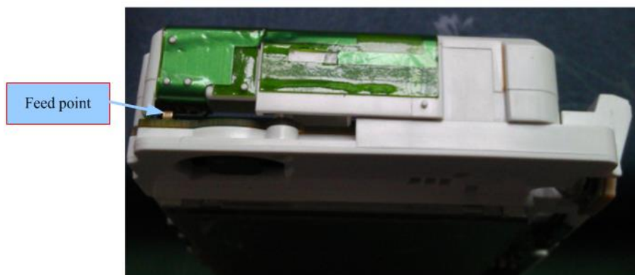
Figure 6: Example of an FPC Monopole Antenna
