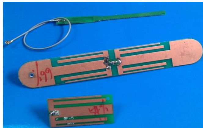
Figure 10: Example of PCB Antennas
