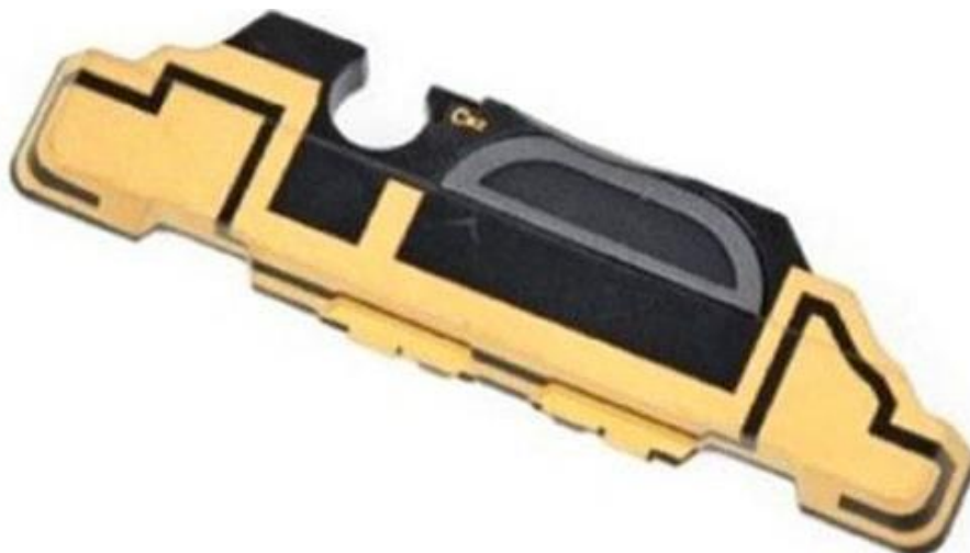
Figure 13: Example of a Laser Direct Structure Antenna
