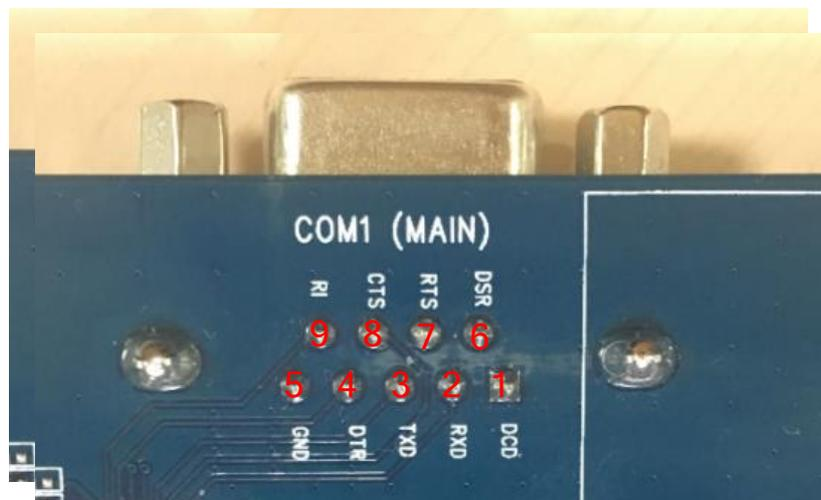
**Figure 25: Pin Assignment of J401**
