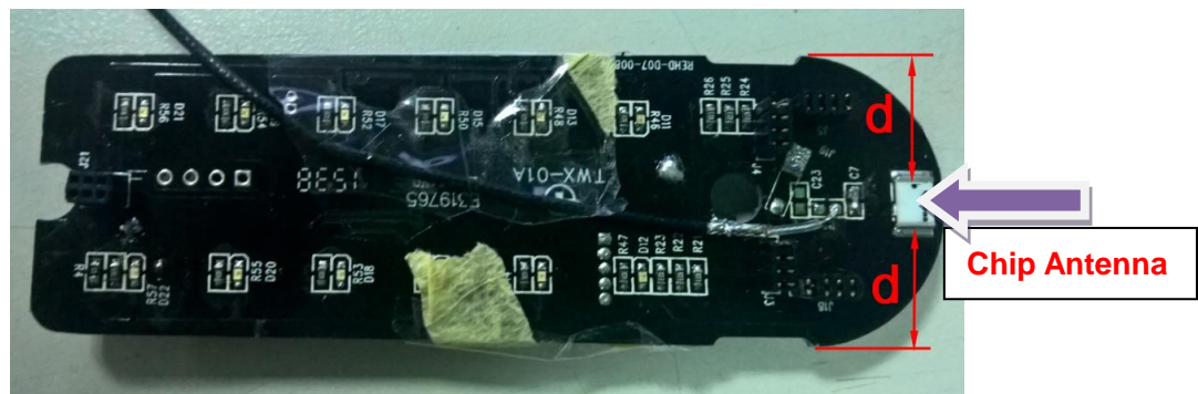
Figure 12: Example of a Ceramic Chip Antenna
