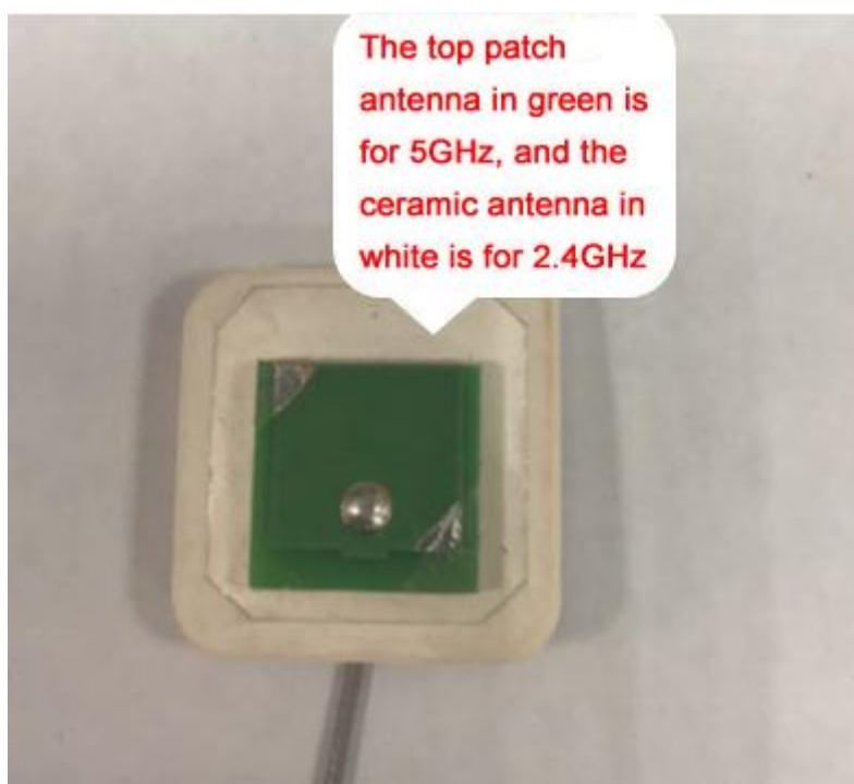
Figure 22: Example of an Embedded Wi-Fi Laminated Antenna
