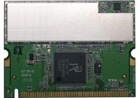
The **WCM6002** is an IEEE802.11a/b/g standard miniPCI card that connects your notebook to a local wireless network. With 802.11a technique, The **WCM6002** can better expand the wireless connection efficiently compared with normal 802.11b/g products.
