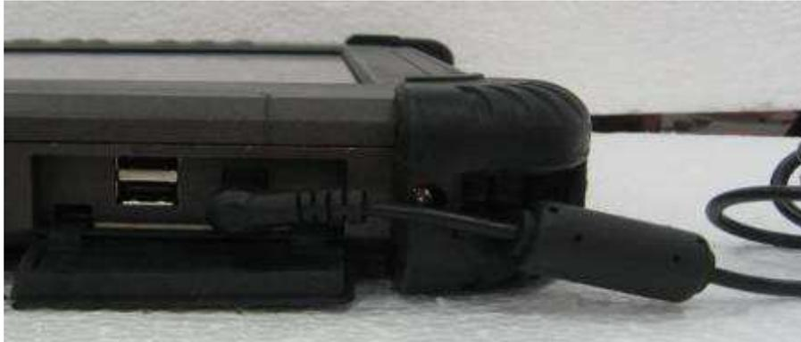
2. By using Multi-functional Docking Station charger, connect power code to the electrical outlet and power connector to the Docking Station. Put battery pack on rear side of charger slot. When the battery is fully charged, the Battery Charge Indicator glows green.
