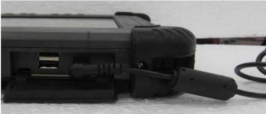
2. By using Multi-functional Docking Station charger, connect power cord to the electrical outlet and power connector to the Docking Station. Put battery pack on rear side of charger slot. When the battery is fully charged, the Battery Charge Indicator glows green.
