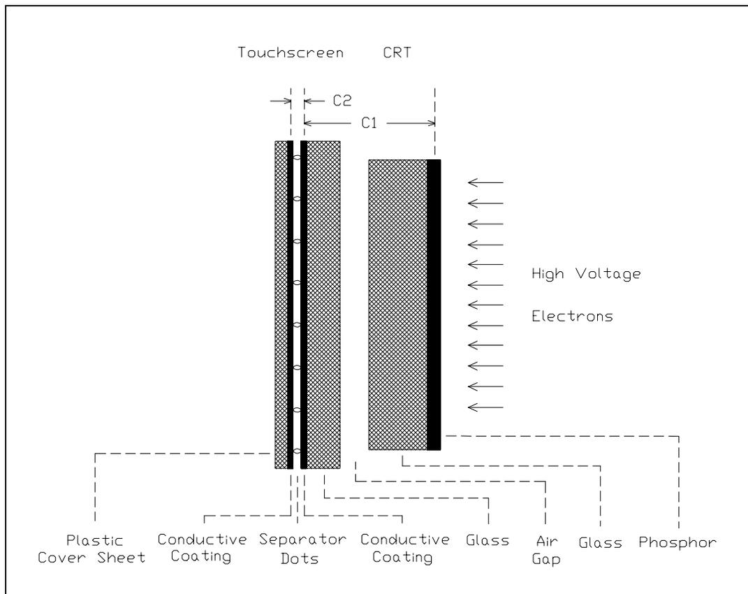
Figure 4-3. Side View of an AccuTouch Touchscreen Installation
