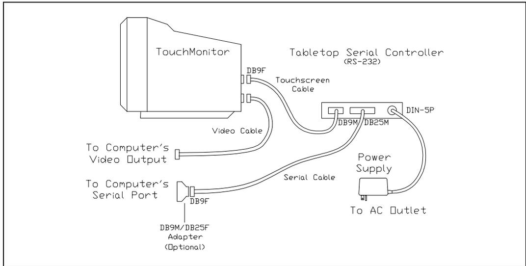
Figure 3-4. E271-2210 Tabletop Serial Controller and Connections
