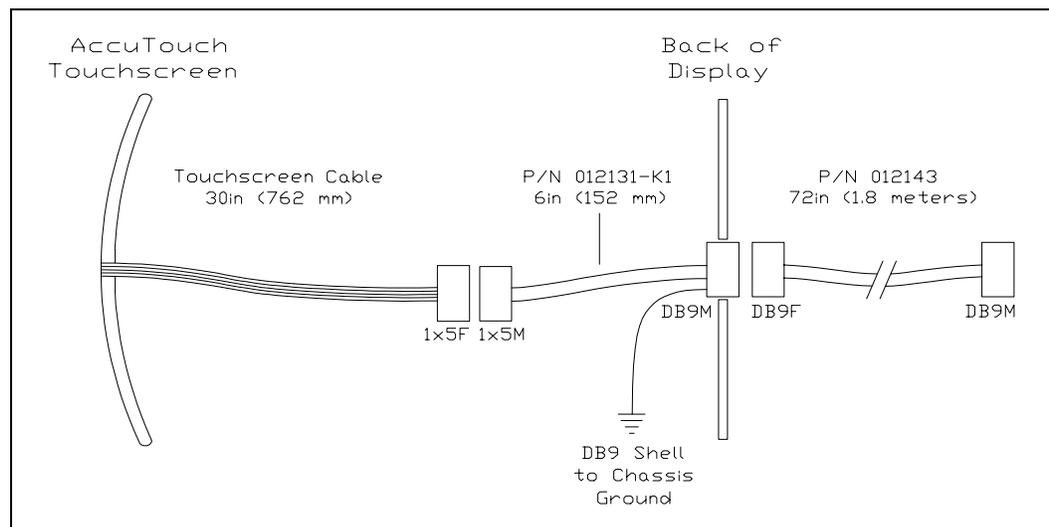
Figure 4-5. Touchscreen Cabling System for External Controllers
