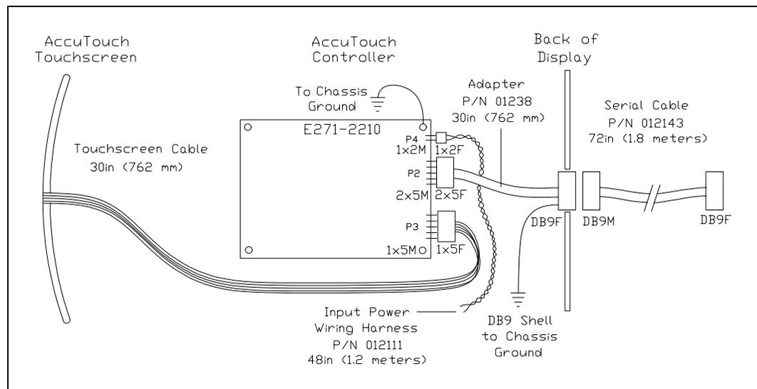
Figure 4-4. Touchscreen Cabling System for Internal Serial Controller
